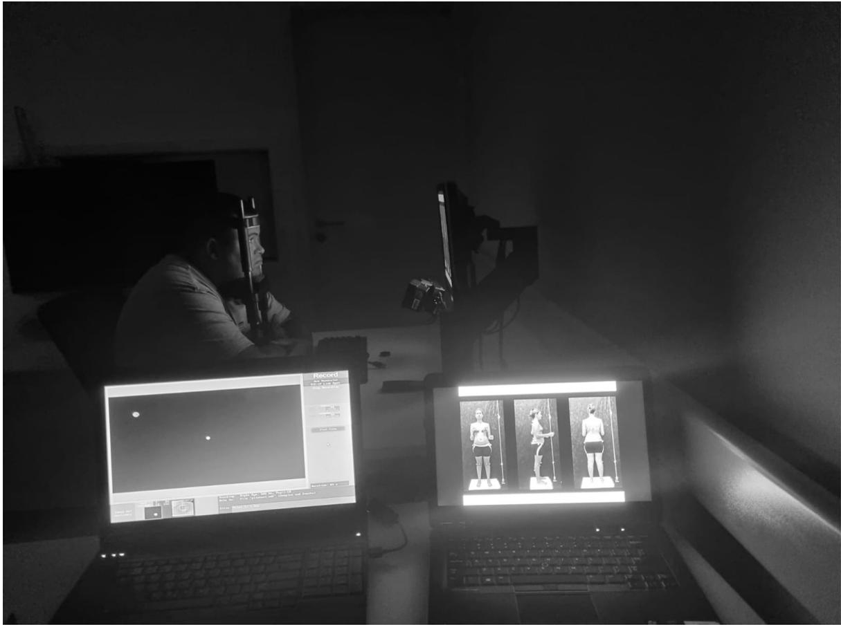
**Figure 1:** Experimental setup for data collection. Seated comfortably, physiotherapists were positioned 60 cm from the eye-tracking screen and instructed to position their face in a head support aligned with the monitor.
